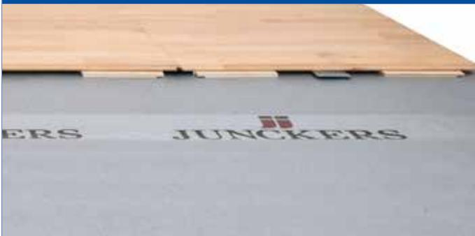
The panels are laid floating over a 5/8" 15 mm sport foam. The intermediate layer of foam is required to provide correct shock absorption and resilience.
