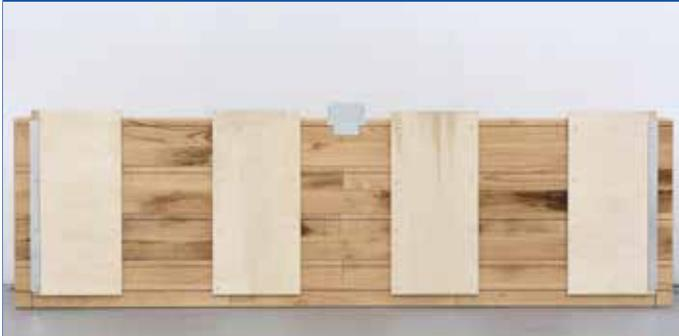
The underside of each panel has four pre-attached 1/2" (12mm) birch plywood support sheets, which improve strength and durability. The panels are further reinforced at each end with "L" shaped aluminum corner profiles.
