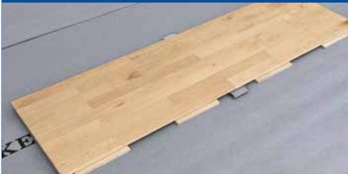
For faster and more flexible installation, Junckers Center Row Panels can be supplied. With metal joining brackets on each side of the Center Row Panel, the installation can start from the center of the floor and work in both directions at the same time.
