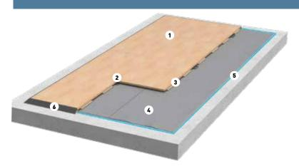
The Arena Master Portable Sports Floor features a 7/8" (22 mm) solid hardwood, prefabricated into lightweight panels.
