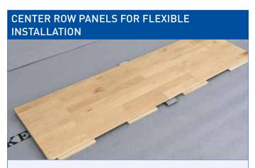
For faster and more flexible installation, Junckers Center Row Panels can be supplied. With metal joining brackets on each side of the Center Row Panel, the installation can start from the center of the floor and work in both directions at the same time.
