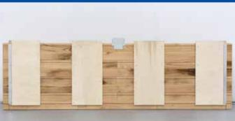
The underside of each panel has four pre-attached 1/2" (12mm) birch plywood support sheets, which improve strength and durability. The panels are further reinforced at each end with "L" shaped aluminum corner profiles.
