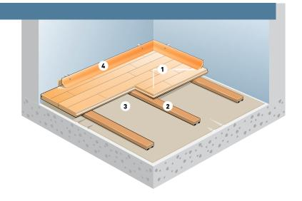
The Unobat 45 System is a low profile, high performance sleeper based system. It is designed for use over flat subfloors.
